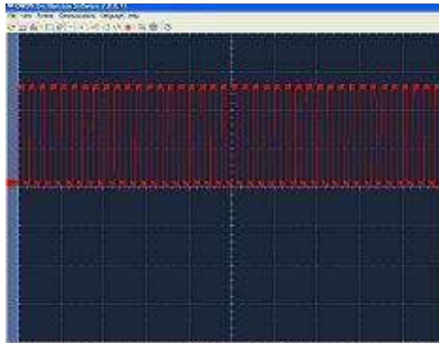
Fig. 20. Waveform at Micro Controller PWM output
